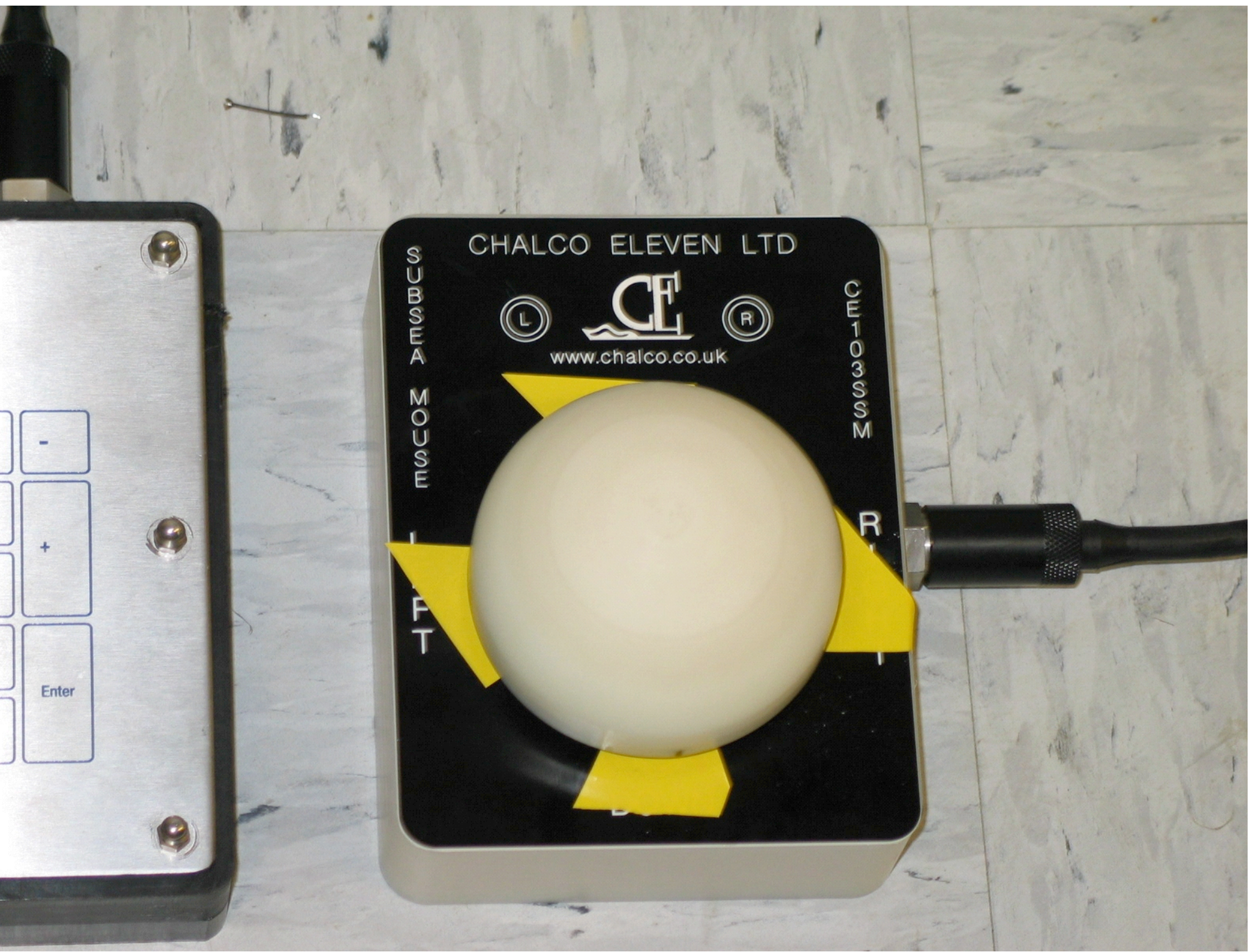
Figure 4. Submersible mouse. The stylus is used on the Left and Right mouse buttons.
