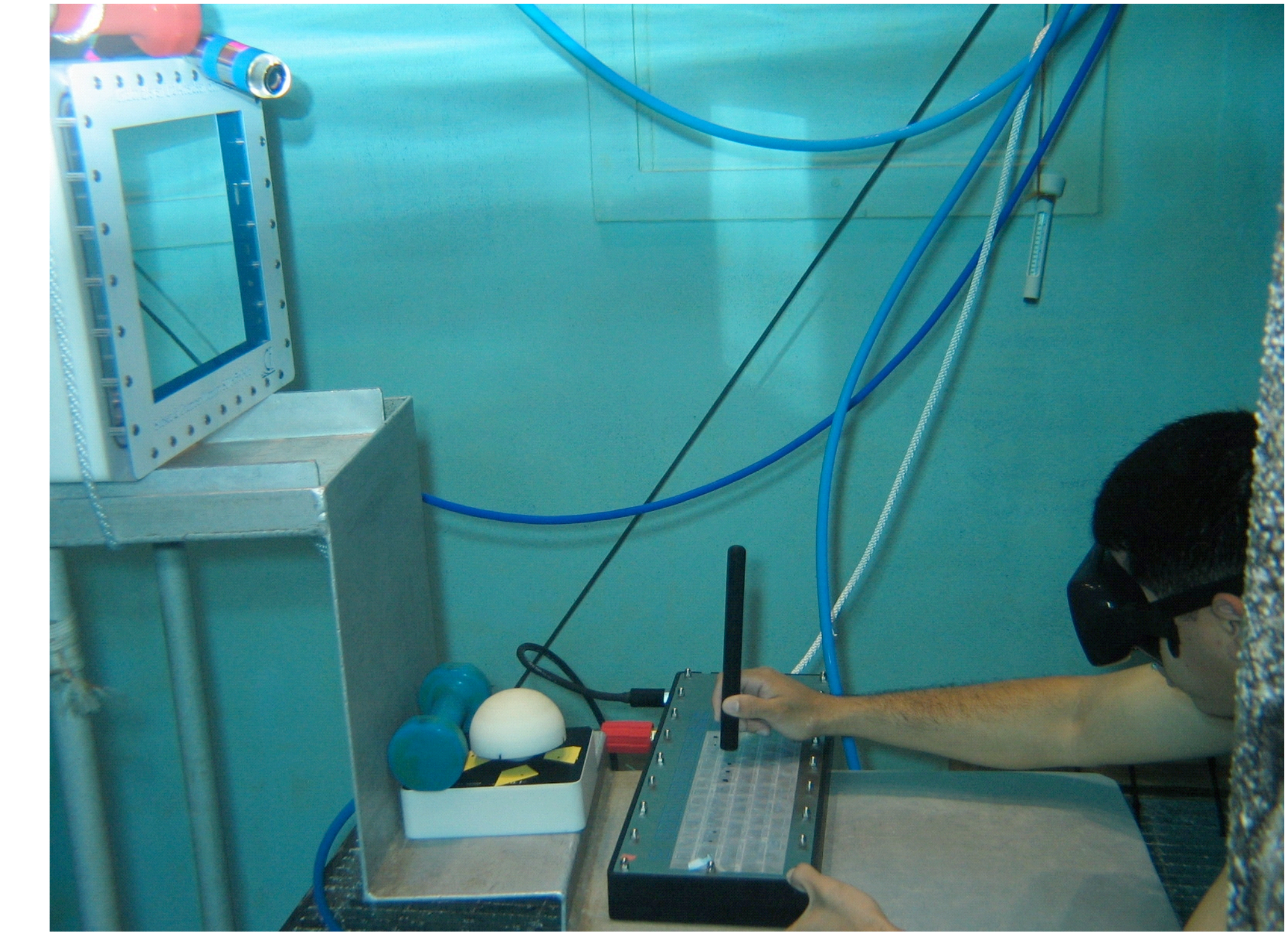
Figure 6. Set up of the submerged monitor, camera, mouse, and keyboard.
