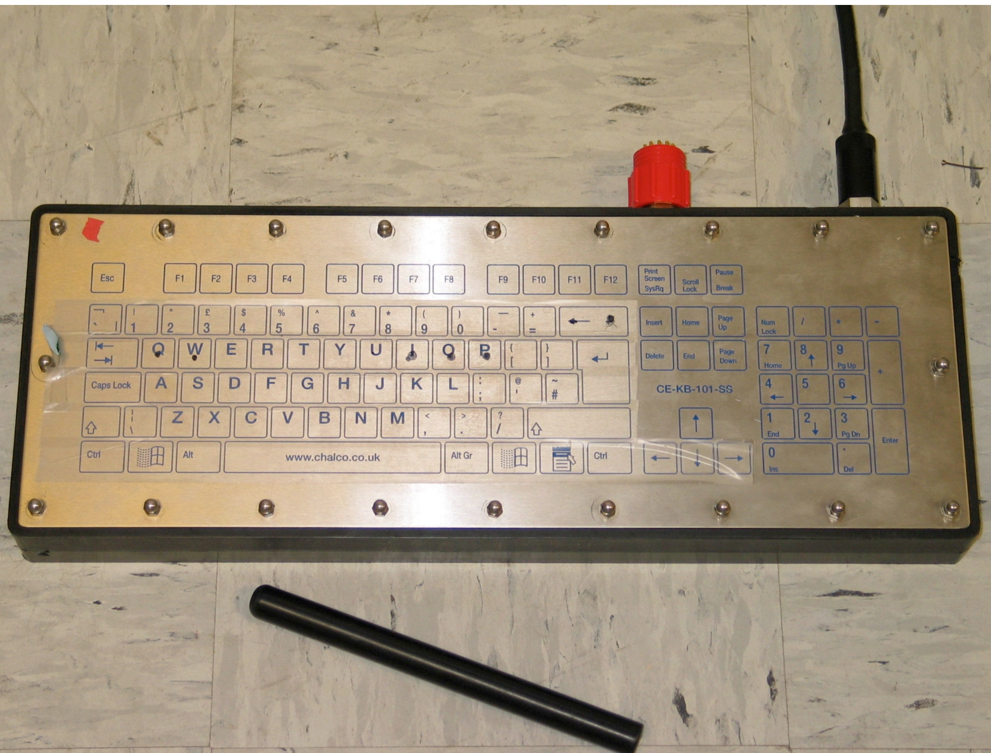
Figure 3. Submersible keyboard and magnetic stylus. This keyboard requires a magnet to operate the keys.
